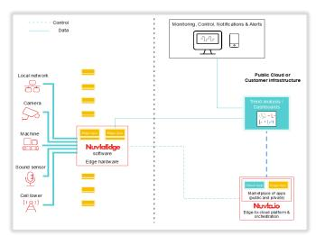
Nuvaled software runs on a range of hardware platforms as small as Raspberry Pi, enabling its integration with IoT sensors at the edge. By establishing a secured connection with the Nuvla.io platform, NuvlaEdge facilitates remote management and real-time monitoring of edge devices, providing teams with enhanced control and visibility over their edge infrastructure.
